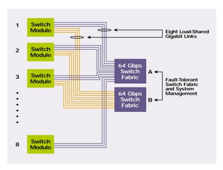
In a BlackDiamond 6808 chassis, a single MSM64i module provides four channels to each I/O slot and each channel is 1 Gbps, full duplex. The addition of a second switch fabric module doubles the number of channels to each slot from four to eight.
