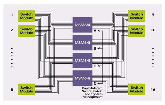
In a BlackDiamond 6816 chassis, a single MSM64i module provides two channels to each I/O slot and each channel is 1 Gbps, full duplex. The addition of three switch fabric modules quadruples the number of channels to each slot from two to eight.
