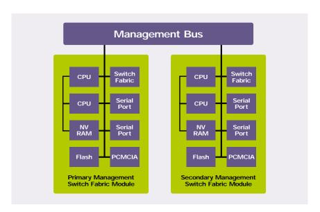
Because the MSM64i modules operate in parallel, one of them must have the role of the master and the others are slaves. The master MSM64i module is responsible for all tasks associated with switch management and protocol processing. This includes running the real time operating system, CLI, ExtremeWare Vista web server, and route processing.
